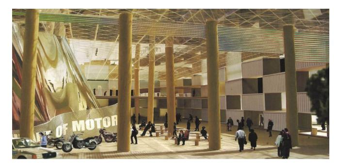
As a temporary structure of at most 10 years was requested, recyclable and reusable materials were used for the building. Paper tubes made of recycled paper were used as columns, and containers were used for the walls and frame structure, covered by a glass roof. A stacking glass shutter façade enabled a smooth transition between the inside and the ocean in front of the building.
