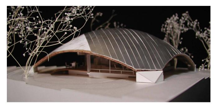
This weekend house is composed of a glass box surmounted by a large woven plywood dome. Four structural plywood boards create the interlocking unit that makes up the woven dome. As the weave is covered by insulation and fiber reinforced plastic, it can be seen only from the inside, similar to ceilings prevalent in traditional Japanese houses.
