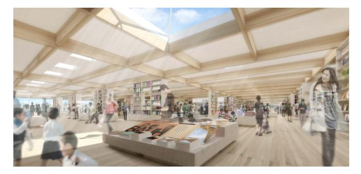
To create a comfortable and homely environment, a timber structure, "house of furniture" is proposed. By providing the required shelving for the bookstore and utilizing these as structure, a column-free, wall-less, and flexible space is realized.
