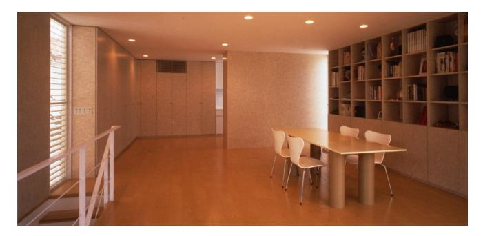
Furniture House 2 is the prototype of a two-story house employing furniture units as structural system. The furniture system used on the first floor is repeated on the second. More furniture units with different functions were developed and combined with "non-furniture" walls to create a system which allowed high flexibility in spatial arrangements.
