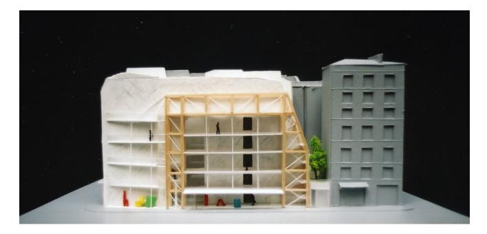
Within the historical "Marais" district of Paris, this apartment building sits on a narrow site flanking an existing fire wall. To minimize disturbance to the wall and to maximize transparency, an independent wooden frame structure was designed to support the suspended floor plates. The openness and flexibility of space is a reaction to the changing lifestyle and working style of Parisians.
