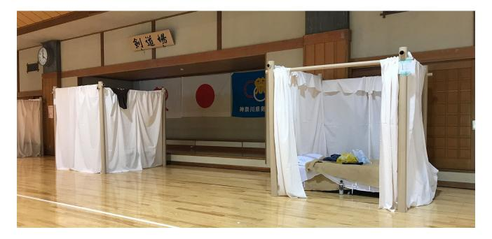
VAN has developed the "Paper Partition System" to be used in order to prevent spreading of virus transmitted through droplets.
