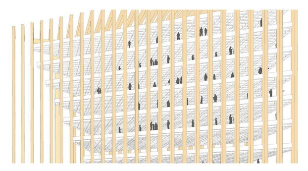
A new Geneva operation center planned for the Médecins Sans Frontières. The Geneva Operational Center will provide work and social spaces for more than 250 MSF staff. An array of timber/steel hybrid portal frames that are rotated 45 degrees against the building grid provides shading against the west sun, as well as air flow throughout the height of the building.
