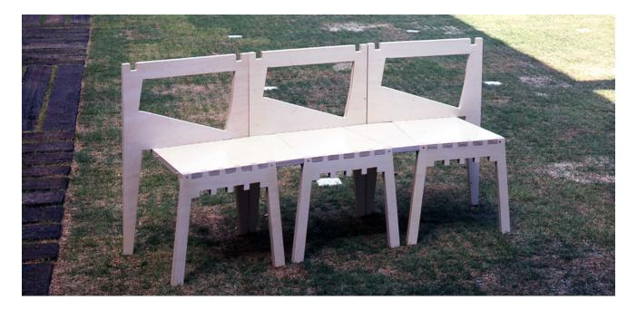
This chair is composed of three cutouts from a single plywood panel; the seat, front legs and backboard. One panel of 900mm  $\times$  1800mm can make three chairs. These chairs are stackable and with a separate piece cut out from the backboard, can be connected to form a bench with a slight curvature, that fits the round space in the church. There are notches cut in the backboard for hanging hand bags.
