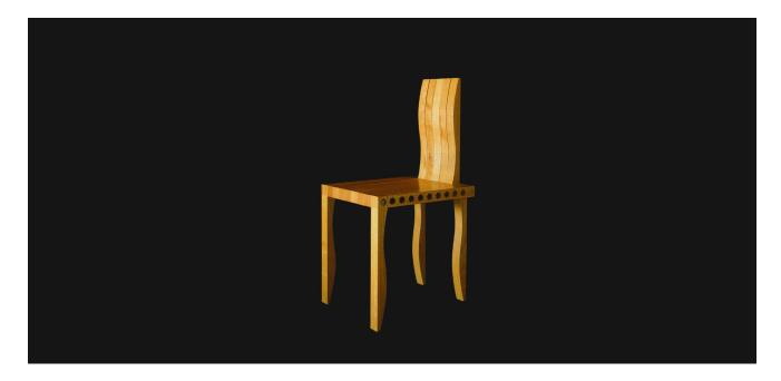
L-shaped units, which pack compactly and therefore ship cheaply, are assembled to compose a variety of chairs and tables. An early prototype made of bent plywood was superseded by the final, solid wood model. Scrap wood from furniture manufacturers was cut to the desired shape and perforated with large holes to reduce weight and to facilitate connections.
