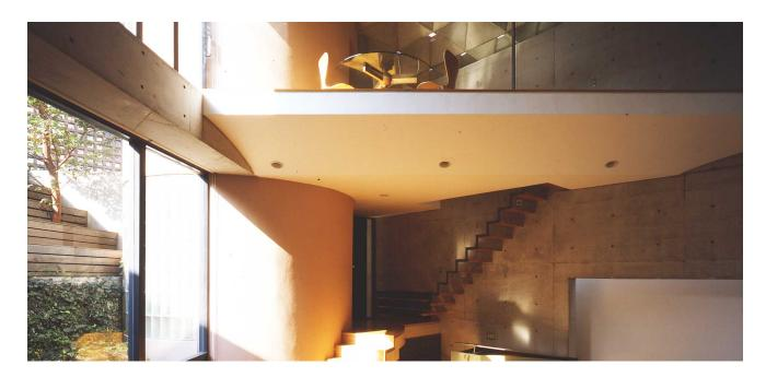
Built in a dense residential area of Tokyo, noise and privacy were considered central design issues for the Studio for Vocalists. The square volume is cut diagonally to separate the interior from an exterior courtyard. A cylindrical and a rectangular core are placed on the diagonal of the building, housing private rooms and wet spaces. A pyramidal waffle slab with skylights roofs a double-story height living room that also functions as a performance space.
