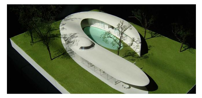
The roof of this boomerang house swoops through the scattered trees, floating in the landscape like an airplane wing in the sky. Ribbed and wrapped with a plywood stress skin, the roof further resembles not only conceptually but also constructionwise the wing of an aircraft. The house sits at the apex of an inlet, and the oval pond situated in the bay of the boomerang creates the illusion of the inlet running into the site.
