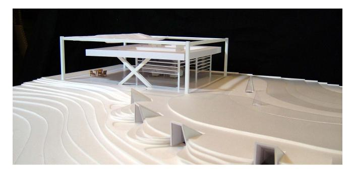
Frequent break-ins during off-season into vacant villas in the resort area of Puglia prompted the client to request a house with advanced security. Mimicking the mechanics of airport container cranes, the roof of the villa was designed to lower completely to the ground, making it impossible to enter when vacant. The glass shutters and furniture can be tucked neatly into the thickness of the roof.
