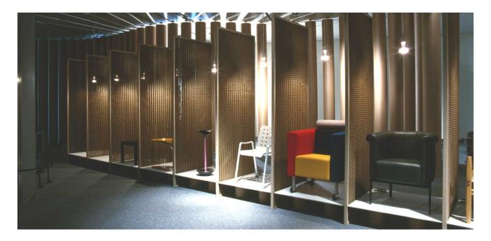
A completely recyclable exhibition system was designed using paper tube walls and square paper tube frames with recycled paper honeycomb infills as partitions.
