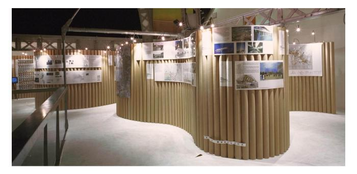
The design for this exhibition required a system which would be flexible and adjustable to travel from one location to another and would provide wall display space of undefined size as well as three spaces for video shows. The wall displays were made of round and square paper-tubes, and for the video spaces aluminium pipes from the previous exhibition were re-used.
