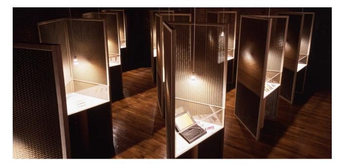
Organized by La Jolla Museum of Contemporary Art in California, the Emilio Ambasz Exhibitions were designed for flexible arrangement and easy global transportation. Square-section paper tubes comprised the frame of the display units, which were made of flat-folding honeycomb screens, while paper tubes of different diameters fitting into each other served as legs for the model stands.
