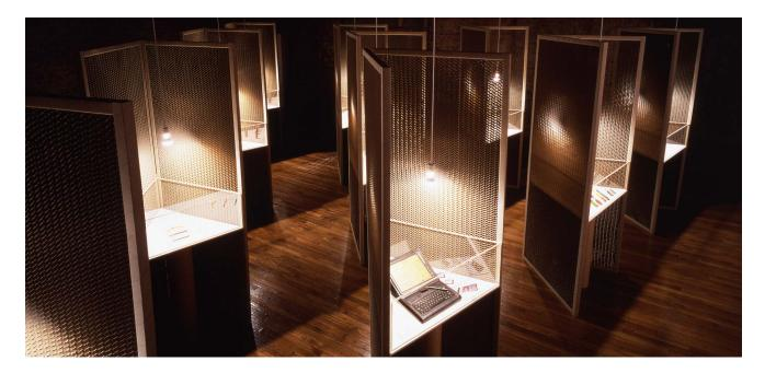
Organized by La Jolla Museum of Contemporary Art in California, the Emilio Ambasz Exhibitions were designed for flexible arrangement and easy global transportation. Square-section paper tubes comprised the frame of the display units, which were made of flat-folding honeycomb screens, while paper tubes of different diameters fitting into each other served as legs for the model stands.
