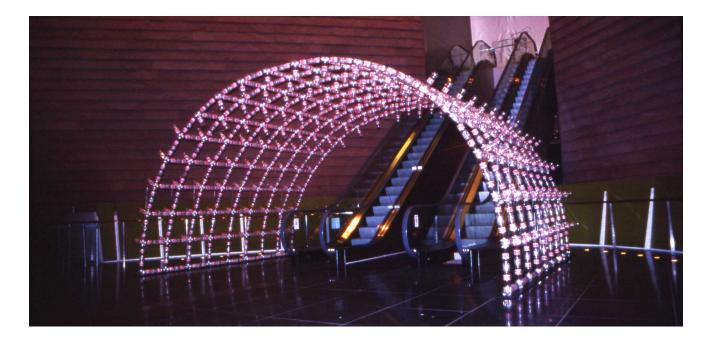
For an exhibition at the Mori Art Museum in Roppongi Hills, plastic bottles were used structurally in order to create an arched entrance gate. The bottom ends of the bottles were taped together to create a uniform member and the cap ends were connected together with an acrylic joint. Because the structure naturally is weak against external loads, the arch was limited to interior use only.
