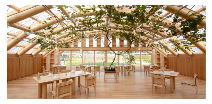
This greenhouse is composed of arches made from paper tubes connected by metal joints. on the exterior, a ready-made greenhouse frame was installed with a double layer of fluorine film with an air layer in between to suppress the temperature changes of the interior. In summer, the leaves of the plants grown inside will cover the ceiling, blocking sunlight.
