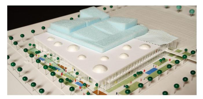
The design of this commercial building, primarily a cinema complex, unifies diverse leisure facilities into one establishment. By making the movie theaters the structural core of the building, the space on the periphery is able to remain light and open with operable glass shutter facades. This peripheral buffer zone imitates traditional Japanese architecture by creating an inviting, intermediate public space.
