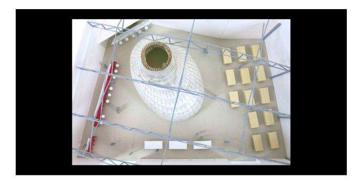
The aim of this project is to accommodate new functions inside the existing Camper factory located in Mallorca. In the middle of this space, a paper honeycomb structure is designed to host the main store. This structure of nine meters height is covered by Tyvek Paper and during the night creates a "lantern" effect thanks to the spotlights integrated into the shelves. Additional spaces, like workshops and a bar surround the structure.
